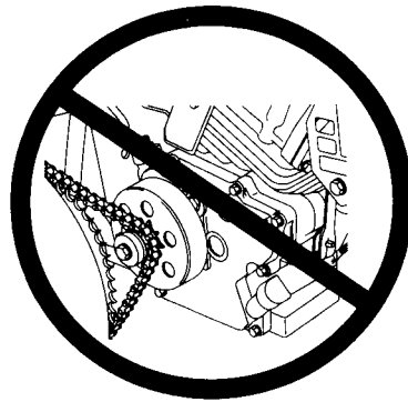
Figure 1. DO NOT use Without Engine Shaft Guard
